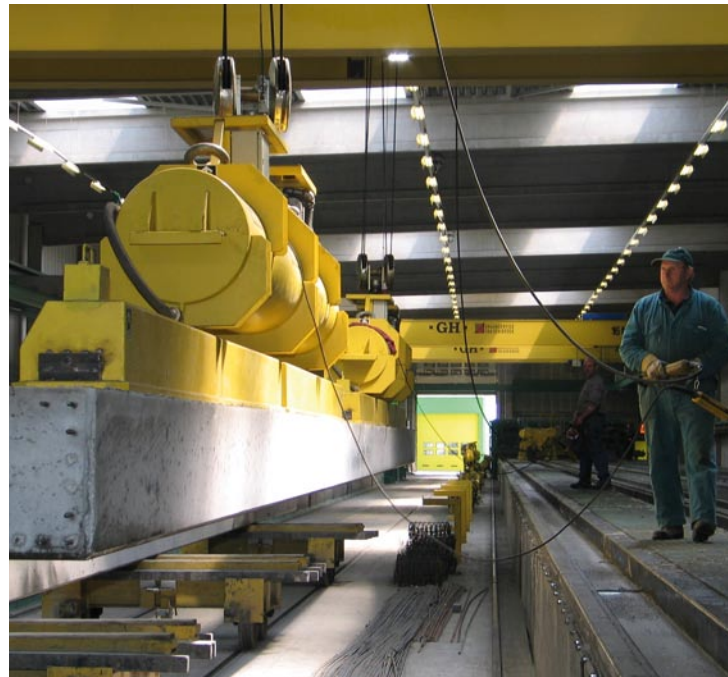
Precast concrete elements are factory made under strict controls. The manufacture of structural elements is automated to a considerable extent. Courtesy of British Precast and Bond van Fabrikanten van Betonproducten in Nederland (BFBN).
