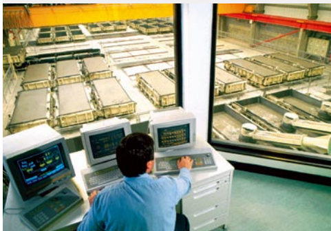
Precast concrete elements are factory made under strict controls. The manufacture of structural elements is automated to a considerable extent. Courtesy of British Precast and Bond van Fabrikanten van Betonproducten in Nederland (BFBN).
