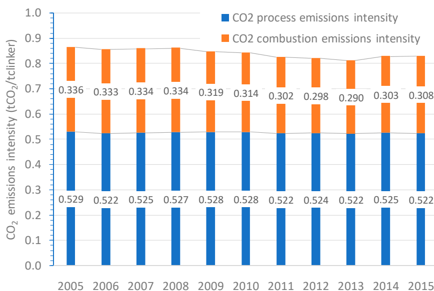
Figure 12. CO 2 global emissions intensity (tCO 2 /t clinker ). Evolution from 2005 to 2015 of the Spanish clinker production.
